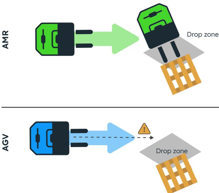
AMRs make use of detection – that is, positive confirmation via on-board sensors – to determine if the pallet is there before they attempt the pickup. If the pallet is askew, or slightly out of the drop zone, the robot will be able to identify it. If the right pallet is not where the AMR anticipated it should be, it will move to the next drop area and search again.
