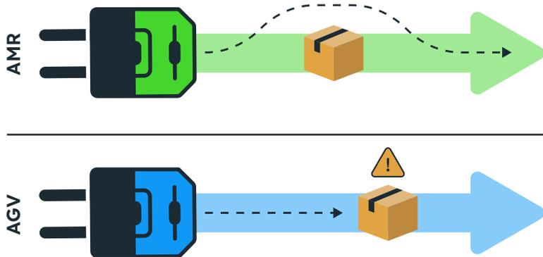
Path Planning allows an AMR to adjust routing and navigate independently around obstacles without stopping and requiring assistance from workers.
